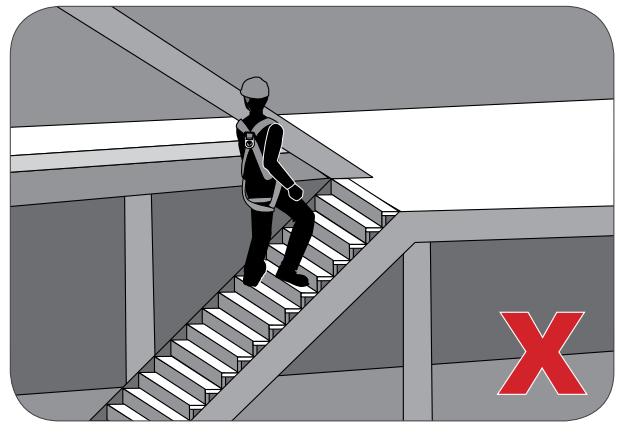
Figure 6.2: Unprotected stairways pose a falling hazard.
