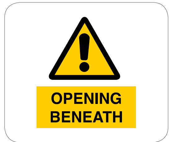
Figure 6.8: A warning sign can be affixed to the opening cover or placed near a barricaded opening.
